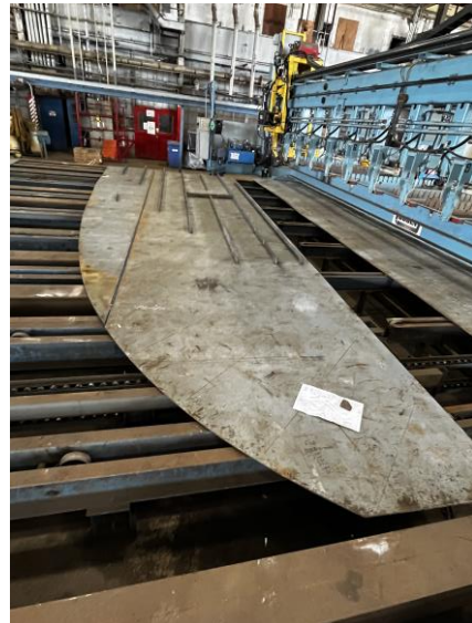
2957 – Starboard Main Deck plating for Module 5
