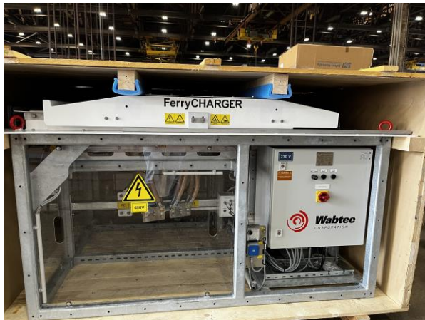
3258 – Charging Socket for the shoreside charger
