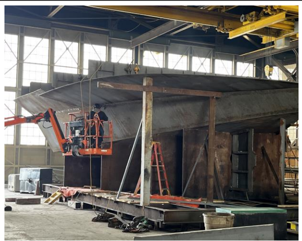
2978 – Module 1 with more hull plating being added
