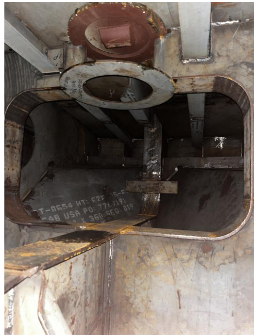
4895 – Rudder Post Tube from Lazarette
