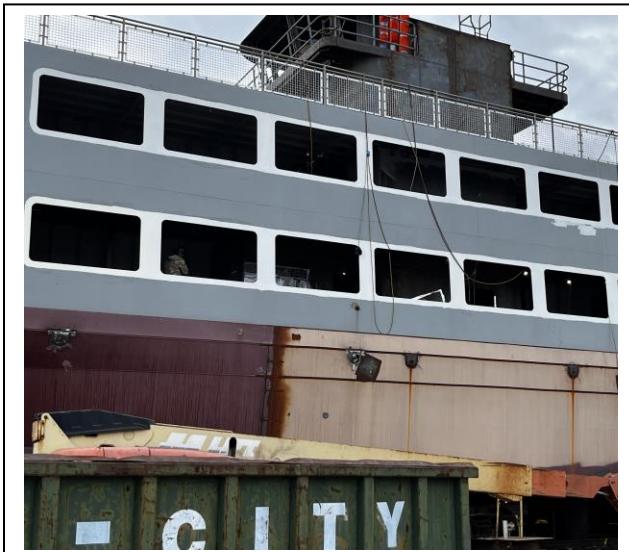
4953 – Paint Prepping Around Windows for Window Installation
