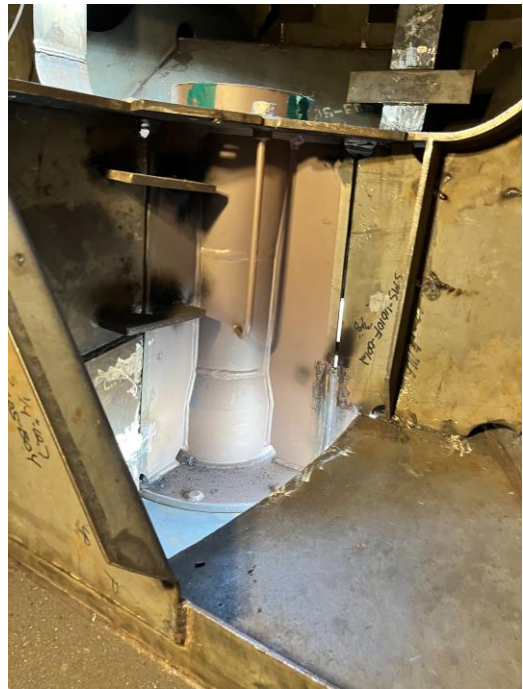
5050 – Rudder Post Tube from the Lazarette
