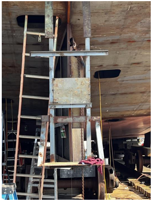
4882 – Aligning Stern Tube Before Welding
