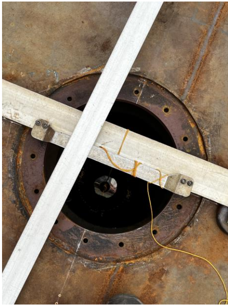
4957 – Aligning Rudder Post Tube
