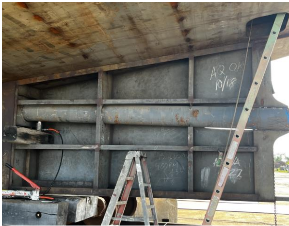
4883 – Aligning Stern Tube
