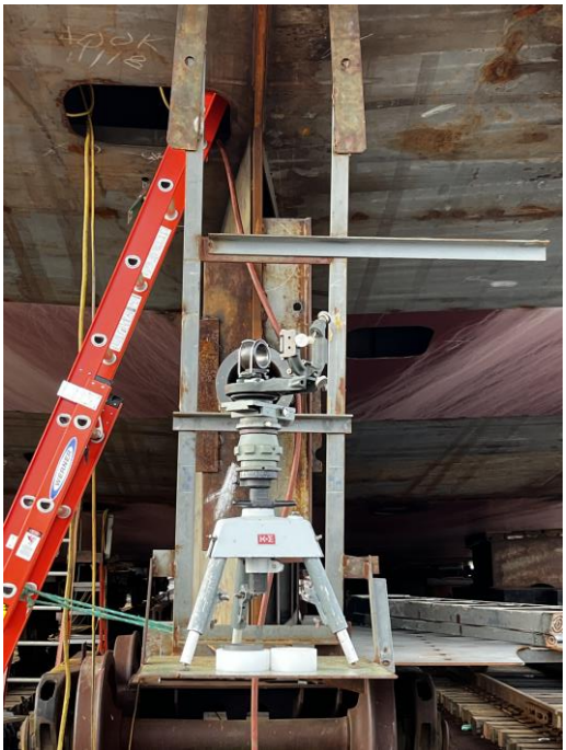
4849 – Aligning Stern Tube
