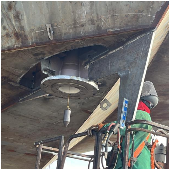
5038 – Aligning Rudder Post Tube and Shroud
