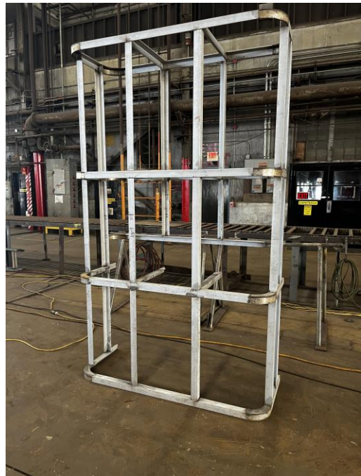
4928 – Heat Sheild Frame for Exhaust Piping
