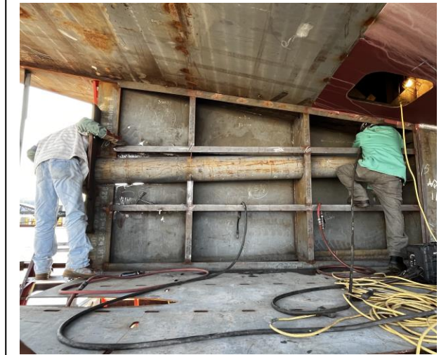
4869 – Working on a Stern Tube
