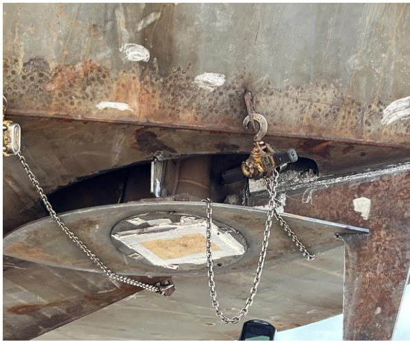
5048 – Aligning Rudder Post Tube and Shroud
