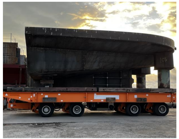
3353 - Module 1 Heading Towards the Assembly Area (Erection Yard)
