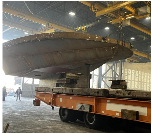
3439 - Module 5 Being Loaded onto the Trailer to be Moved to the Assembly Area
