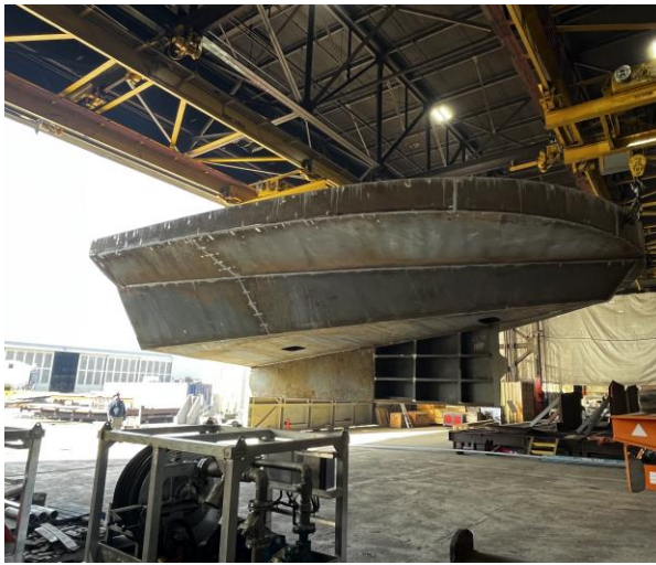
3343 – Module 1 (Bow End) Lifted and Ready to be Loaded on Trailer
