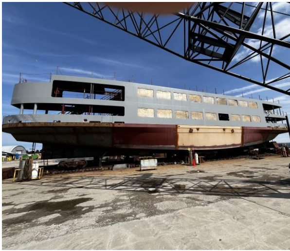
4377 – Super Structure Starboard Side – Next Paint Coat
