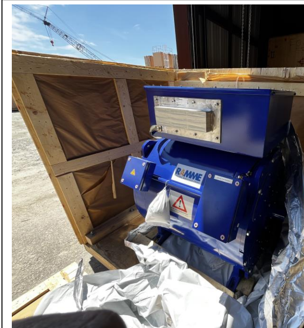
4417 – Electric Propulsion Motor
