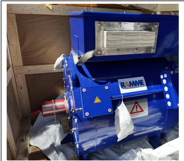
4415 – Electric Propulsion Motor
