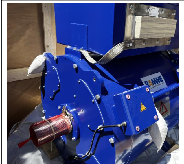
4420 – Electric Propulsion Motor
