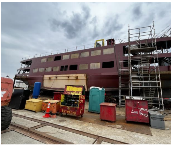
4321 – First Coat Paint on Port Side
