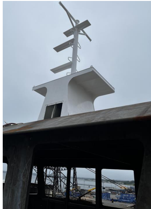
4765– Mast on Pilot House
