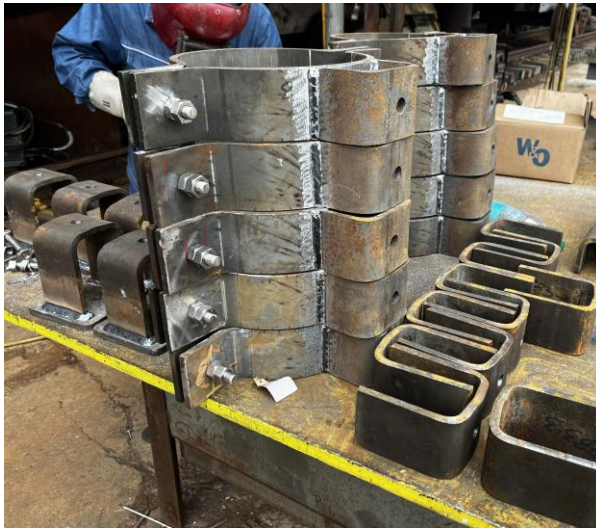
4762 – Piping Clamps & Supports
